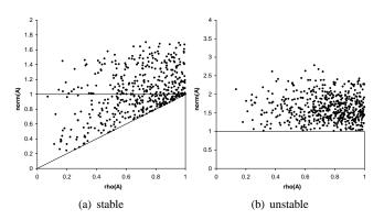
Fig. 3. Delayed stability as a function of  $\rho(A)$  and  $||A||_2$ .
