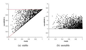
Fig. 4. Delayed stability as a function of  $\rho(A)$  and  $\inf_{W} ||WAW^{-1}||_2$ .
