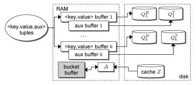
Fig. 1. Operation of DRUM.
